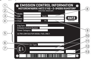
The engine type plate is affixed to the air guide housing and includes the following engine information:
