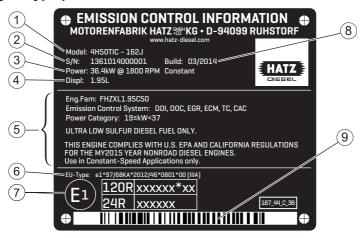
The engine type plate is located on the crankcase and contains the following engine information:
